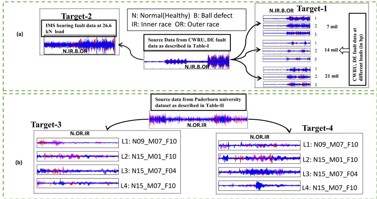
Fig. 5. Domain change from source to target for the two cases. (a) Source and target datasets as described in Table I. (b) Source and target data as described in Table II (the waveform in red, blue, and magenta colors is the vibration signals).
